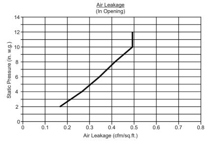
Air leakage chart is based upon independent air leakage tests conducted by Architectural Testing Laboratory. The out-opening model of a 26" x 60" AHF-T2I was tested. Tests were in accordance with ASTM E 283-91 "Determining the Rate of Air Leakage through Exterior Windows, Curtain Walls, and Door under Specified Pressure Differences Across the Specimen". Air Balance recommends using out of opening doors for draw through applications and in opening (IO) for blow through applications.
